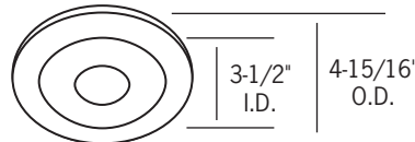
CTR2011-PH-(NK, P) Flat Frosted Glass Lens Shower Light with Clear Pin Hole All steel construction. (3) heat treated spring steel mounting clips. 1/8" thick heavy duty polyethylene sponge gasket. Wet location listed.
